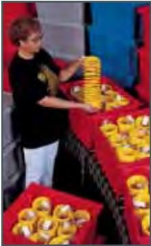
Nest & Stack Totes stack when full; turn 180° and nest when empty.
