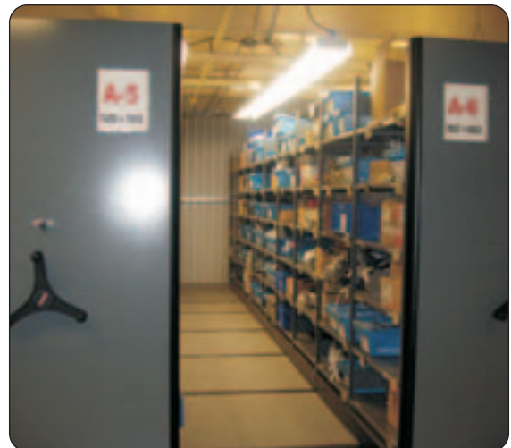
MECHANICAL-ASSIST MOBILE AISLE SYSTEMS CAN BE DESIGNED WITH INDIVIDUAL CARRIAGES UP TO 36 FEET LONG.
