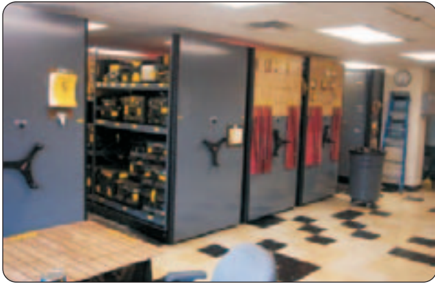
MECHANICAL-ASSIST END PANELS ARE DESIGNED FOR HANGING FREQUENTLY ACCESSED ITEMS TO ENHANCE THROUGHPUT.
